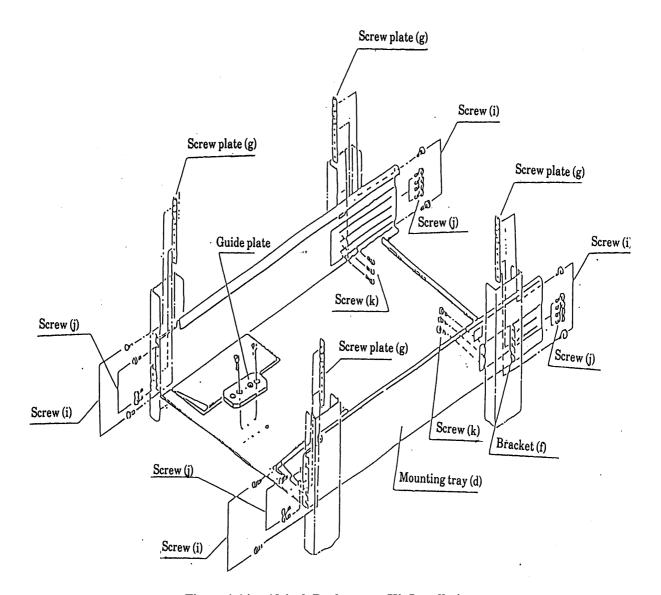
Figure 1-14. 19-inch Rack-mount Kit Installation
